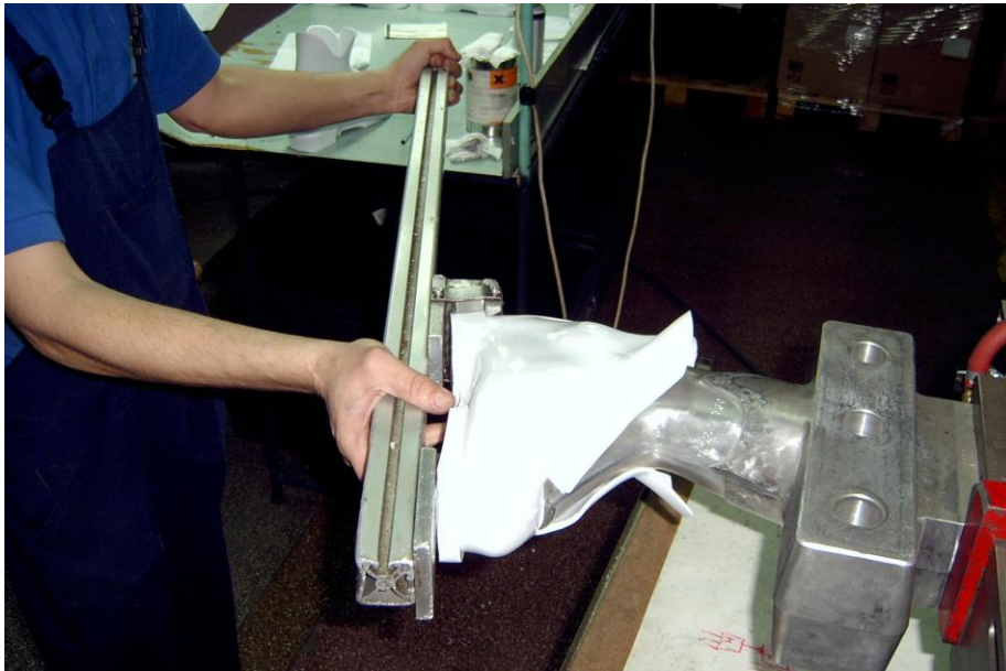
Picture 4. Manual extraction of the inferior body of a alpine ski boot
